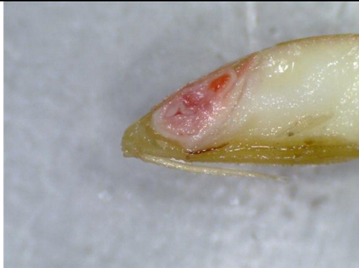
Image 11: Very weak staining – fail (in reference to other grains)
