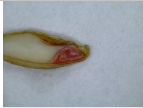
Image 10: Even staining, but not strong – pass (in reference to other grains)
