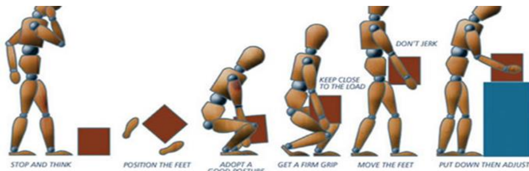
Diagram shows correct lifting technique.
